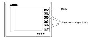
When a key is pressed, the HMI will make a "beep" sound to signal that a command is pressed. (The default setting is a 200 ms beep, and can be configured.)
