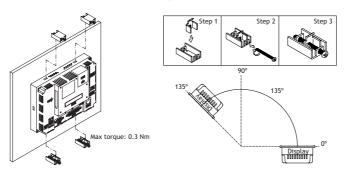
3. The HMI must be installed within an angle of 0° to 135° as shown above.
